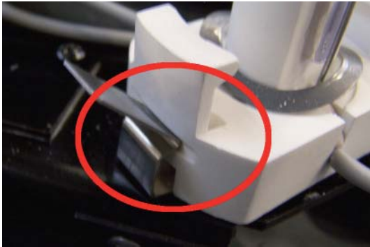
Figure 45.1: Inserting the new sunlamp so that it fits precisely
