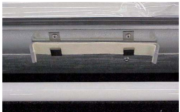
Figure 40.4 Hooks for attachment of bed pane
