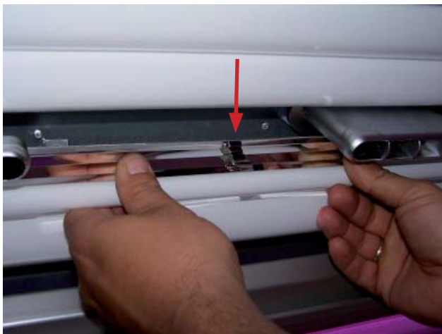
Figure 43.2: Centre retaining clamp of a P2 tube
