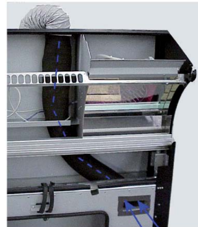
Figure 48.3: Cold air for the canopy (assembly picture)
