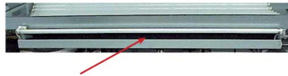
Figure 47.3: Filter pad in the base section
