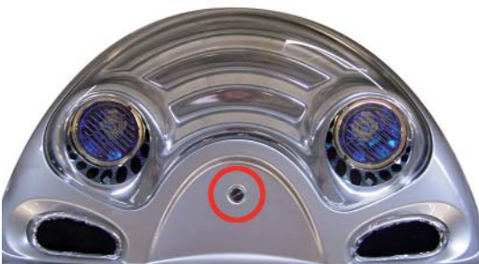
Figure 44.1: Undoing the screw of the outer covering
