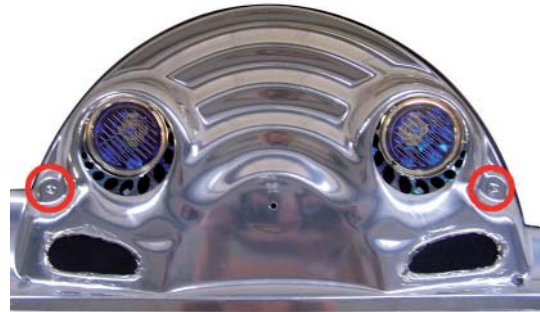
Figure 44.3: Disconnecting the reflectors from the power supply at the respective ignition device
