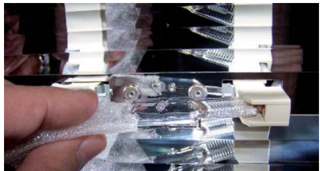
Figure 45.5: Pull out the light bulb towards the front
