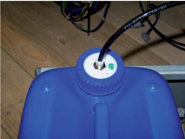
Figure 52.1 Hose connection on aquaCool canister
