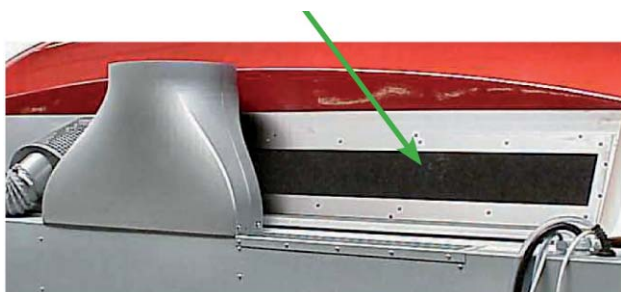
Figure 47.2: Filter pad in the canopy
