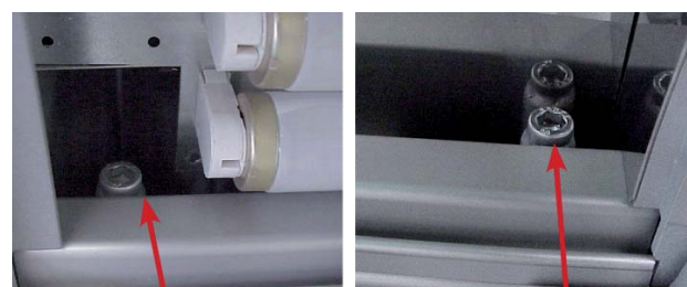
Figure 47.4: Tensioning spring on the left-hand side
