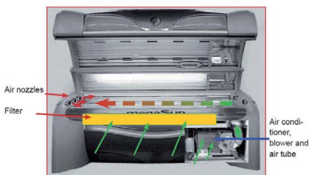
Figure 49.1: Principle of the bed cooling
