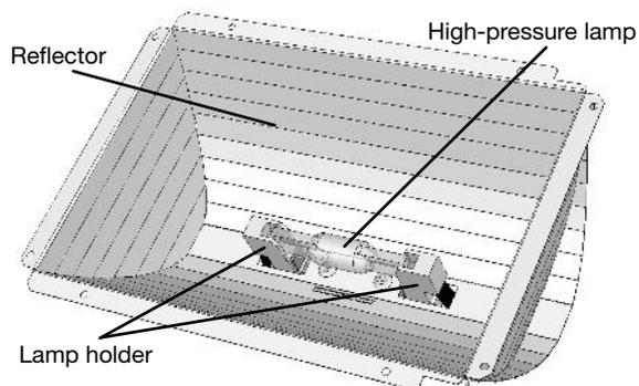
REPLACING THE HIGH-PRESSURE LAMP
