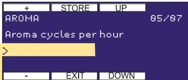
For interval operation of the cabinet scent released, the number of scent releases per hour can be set here.
