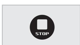
Press <STOP> 2x to cancel the parameter selection and to exit the configuration mode. The standby message "LUXURA, IT'S YOUR BODY" will appear on the display.
